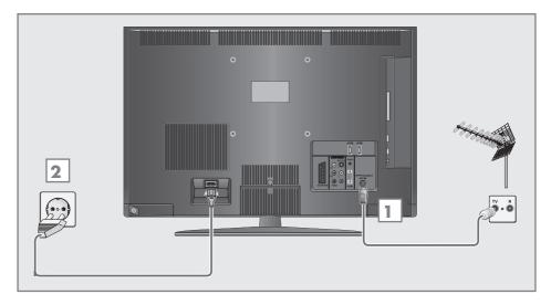
1a To receive terrestrial digital broadcasters (DVB-T) connect the cable for the rooftop or indoor antenna (passive or active indoor antenna with its own power supply) to the antenna socket »ANT IN« on the television set;
